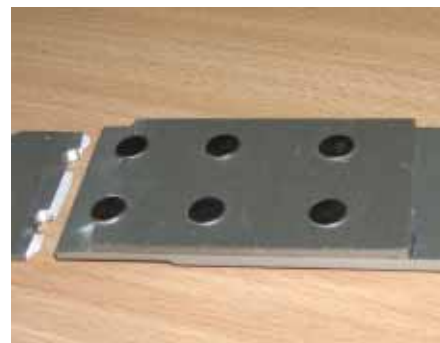
Fig. 2. Specimen after tensile loading
